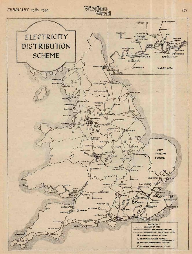
The "National Grid" which will eventually supply power at the standard frequency of 50 cycles to electrical undertakings, combining the various schemes drawn up by the Electricity Commissioners and approved by the Central Electricity Board. The East Anglian scheme still awaits the approval of the Board.
