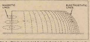
Fig. 1.—Simple inverted "L" aerial showing how the electrostatic and magnetic lines of force are disposed when an oscillating current is flowing. The fields are alternating and one is passing through zero when the other is at maximum.
