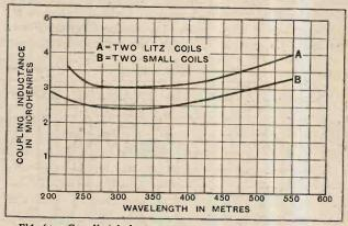
Fig. 6a.—Coupling inductance required for 8 kc. peak separa-tion in filter composed of two Litz coils in the case of A, and two small colls in the case of B. The circuit is that of Fig. 4 (a) or 4 (b).
