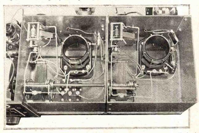
Units 3 and 4. By means of wooden blocks the tuning coils are elevated away from the metal base of the containers. The piece of 1/8in. square metal which gangs the switches is lobsely mounted in the square holes provided so that no trouble is experienced due to errors in alignment,
