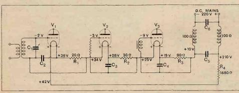
Fig. 1.—With valves series connected the difference in potential across resistances shown at  $R_1$ ,  $R_2$  and  $R_3$  provides grid bias.
