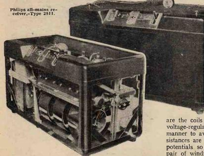
sections being arranged concentrically. Three pairs of short-circuiting blades are used for wave changing. and the metal arms with which these blades make contact are operated from a single lever, which also introduces the gramophone pick-up circuit into the grid of
