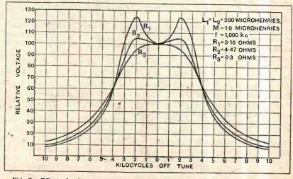
Fig. 2.-Effect of coll resistance on resonance curve of filter. As the resistance is increased the filter behaves more and more like a single tuned circuit.
