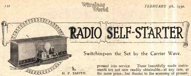
HIS piece of apparatus is intended for connection to an existing detector-L.F. receiver, which is normally tuned to the transmission of a local station. Its function is to switch on the filament current when the station begins to emit its carrier wave, and to
