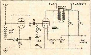
Fig. 1.—Circuit diagram of the relay unit, connected to the grid circuit of a receiver (shown in dotted lines). C, 0.0002 mfd.; C<sub>1</sub>, 2 mfds.; R, variable resistance, 400 ohms; R<sub>1</sub>, 25,000 ohms; R<sub>2</sub>, 50,000 ohms; R<sub>3</sub>, lamp resistance, 2,000 ohms; R<sub>4</sub>, 2 megohms.
