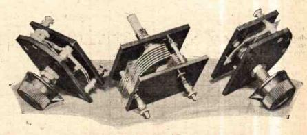
"Omnivox" variable condenser with "Acetoloid" solid dielectric.
