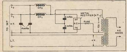
Fig. 2.-Circuit details of a metal rectifier using the voltage-doubling bridge scheme.
