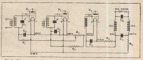
Fig. 2.—When a tapped resistance  $(R_3)$ , provides grid bias for two or more values, decoupling of the grid circuits is desirable.  $R_1$  and  $C_2$  decouple  $V_1$ , and  $R_2$  and  $C_3$  perform this duty for  $V_2$ .
