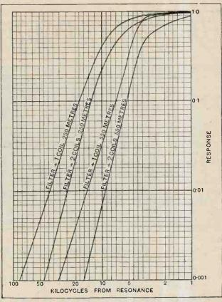
Fig. 12.-Resonance curves of filter using two Litz coils in con-junction with one or two small coils as single circuits.
