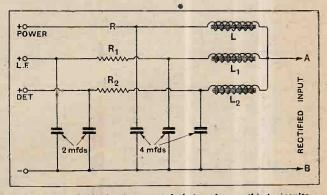
Fig. 5.—Individual voltage-regulating and smoothing circuits for connection direct to a rectifier.
