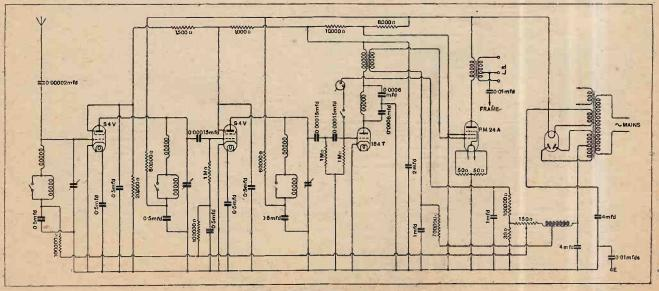
Circuit of Philips four-valve A.C. set.
