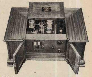
Gambrell 4-valve all-mains D.C. set. Two pentodes are used in parallel as the output stage.
