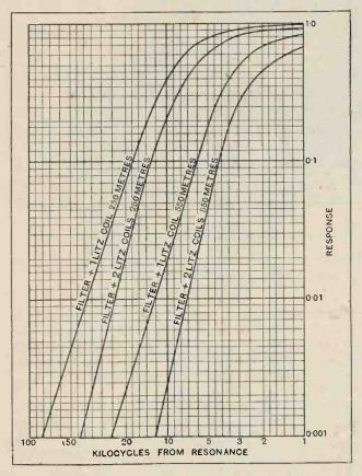
Fig. 11.—Re:onance curves of filter using two Litz coils in con-junction with one or two Litz coils as single circuits.
