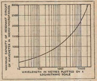
Fig. 7.—Curve from which to find the maximum circuit capacity permissible for a wavemeter of any given order of wavelength.
