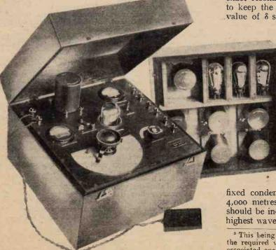
A modern commercial heterodyne wavemeter. Note the cylindrical interchangeable colls.
