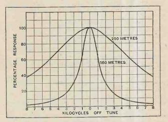
Fig. 8.-Resonance curves of two Litz circuits in cascade, at 250 and 550 metres.
