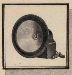
Senior \* R.K." Unit with A.C. Field Excitation. Tids "R.K." Upit has a 10in. corru-gated cone with moving coil, having an impedance of 10-15 ohms at 50/4,000 cycles. The pot magnet is mounted in a pressed metal base, which also con-tairs a mains transformer, Mazda U.U. 60/256 rectifier vaive, and smoothing con-denser for the supply of field current. Price £11/10/0.
