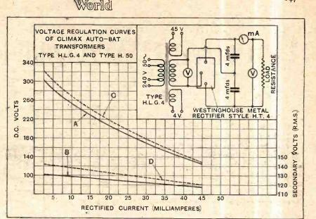
Voltage regulation curves of Climax Auto-Bat transformers using a Westinghouse H.T.4 rectifier. A, the rectified output and B, the secondary voltage regulation of H.L.G.4 model. Curves C and D are the rectified and A.C. outputs from the H. 50 model.
