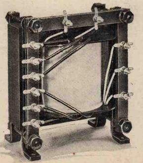
View of the finished 25-cycle transformer.
