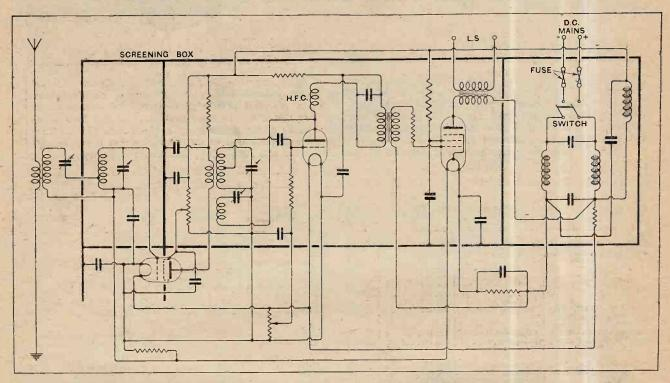
Fig. 4.--Suggested scheme for a 3-valve all-electric D.C. set. Complete screening of the eliminator is advocated, and an input filter, with aerial fully insulated, as shown. The H.F. and detector filaments are in parallel but in series with the pentode. The container is not "live," and may form the cabinet.
