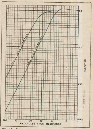
Fig. 10.-Resonance curves at 225 and 550 metres of filter consisting of two compact 2in. coils coupled by 2.50 microhenries.
