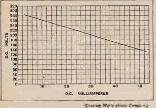
Fig. 2.—Voltage output of the eliminator shown in Fig. 1 (without resistance R) under varying loads.
