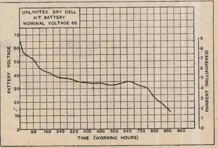
Discharge curve of the "Unlimitex " 60-volt battery.
