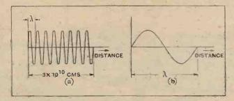
Fig. 3.—(a) Radio waves travel with a speed of  $3 \times 10^{10}$  cms. per sec. When the frequency is f cycles per sec. f waves occupy a space of  $3 \times 10^{10}$  cms. (b) One wavelength  $\lambda = \frac{3 \times 10^{10}}{f}$  metres. f
