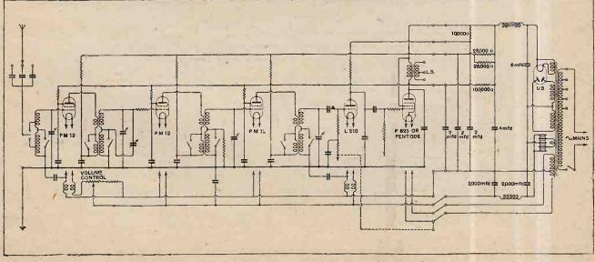
Circuit of Columbia Model 304 receiver with A.C. mains unit.
