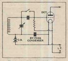
Fig. 1.—Anode bend or leaky grid. A simple switching scheme.
