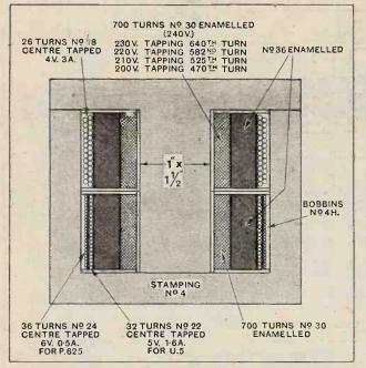
When used with the single P.625 output valve the 36 gauge winding consists of 1,500 + 1,500 turns. Practical hints on the making up of small transformers of this type have been given in recent articles.
