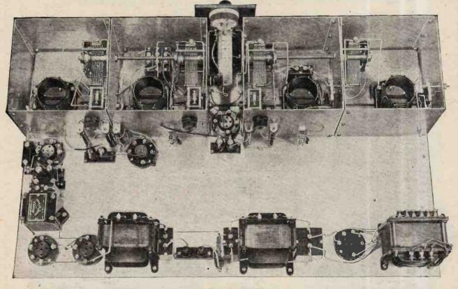
A merit of the home-built set is that it can be easily modified and for this reason a wide baseboard is used which provides space for the later inclusion of additional apparatus.
