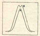
Fig. 1.—A is typical of the overall resonance curve of two tuned circuits that are not directly coupled to one another, but are separated by a valve. B shows the type of curve that arises when there is coupling between the two circuits. In each case, the curve shown is the joint curve of the two circuits taken together.
