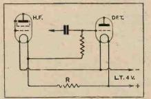
Fig. 1.—A 2-volt H.F. valve with 4-volt valves elsewhere: a form of connection giving 2 volts positive blas for grid de-tection.
