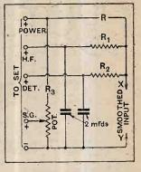
Fig. 4. — Parallel output feeds for connection to similarly lettered points on the nucleus eliminator.
